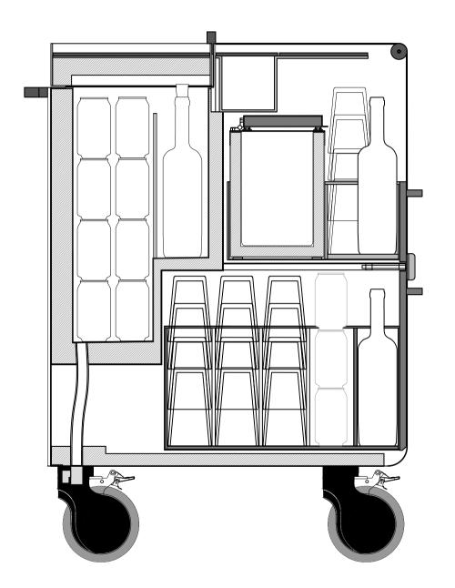
CONSTRUCTION Aircraft aluminum body & frame, stainless steel moldings, roto molded polyethylene cooler & bins
